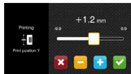
Print position Y Fast setup with a slider, fine setup with \pm keys
